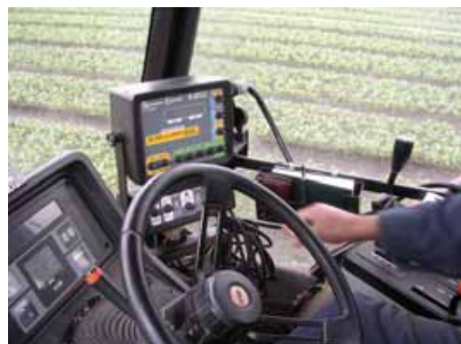
In cabin rate controller
